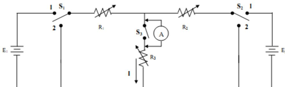
2. Keep both sources active by keeping  $S_1$  &  $S_2$  in the proper position (position 1).
