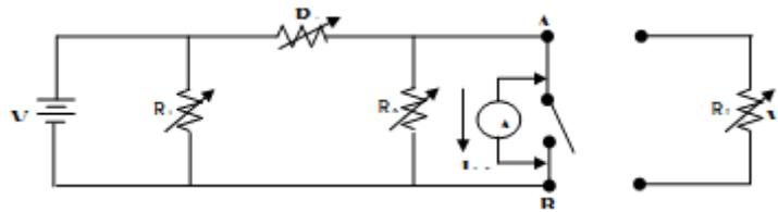
Alternatively find the Thevenin resistance by opening  $R_L$ , disabling the voltage source and measuring the resistance across terminal AB using multimeter and verify that in both cases the resistance is same.
