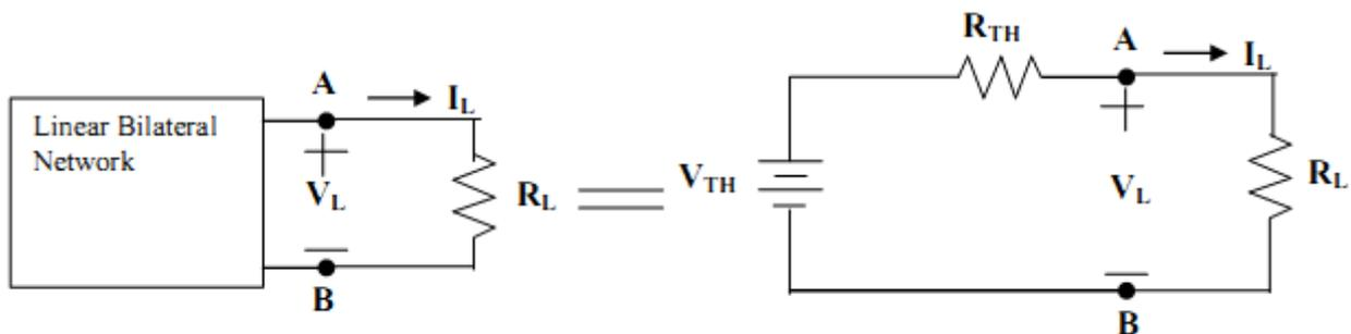
There are several methods for determining Thevenin resistance  $R_{TH}$ . An attractive method for determining  $R_{TH}$  is: (1) determine the open circuit voltage, and (2) determine the short circuit current  $I_{SC}$  as shown in the figure; then
