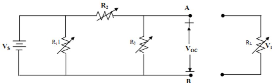
4. Place a short circuit between terminals A & B and find the short circuit current  $I_{SC}$ . Divide the open circuit voltage by the short circuit current to find the Thevenin Resistance  $R_{TH}$  i.e.
