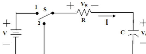
**CHARGING PHASE:** When the switch is connected to position 1, applying KVL we can write
