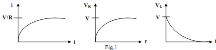
It is seen from the curves that the voltage across the inductor falls from V to zero volts exponentially. The current is zero at the start i.e. when the switch is just thrown to position 1, then it increases exponentially and finally reach to V/R amps when the inductor voltage becomes zero.
