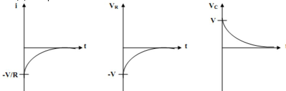
It is seen from the curves that the voltage across the capacitor falls from  $V$  to zero volts exponentially. The charging current is maximum at the start i.e. when the switch is just thrown to position 2, then it decreases exponentially and finally ceases to zero when the capacitor voltage becomes zero.
