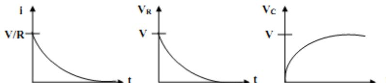
It is seen from the curves that the voltage across the capacitor rises from zero to V volts exponentially and the charging current is maximum at the start i.e. when C is uncharged, then it decreases exponentially and finally ceases to zero when the capacitor voltage becomes V.
