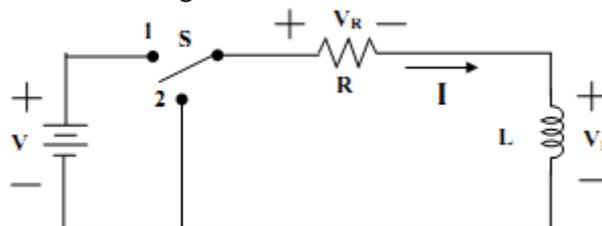
**Storage Phase:** When the switch is connected to position 1, applying KVL we can write
