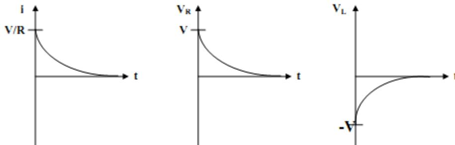
It is seen from the curves that the voltage across the inductor rises from -V to zero volts exponentially. The current is maximum at the start i.e. when the switch is just thrown to position 2, then it decreases exponentially and finally ceases to zero when the inductor voltage becomes zero.
