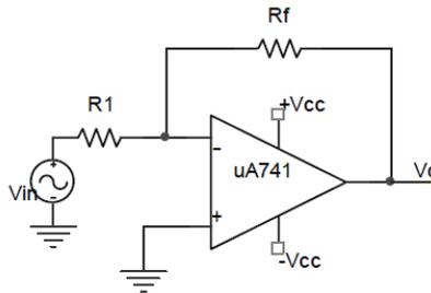
Figure 3 Inverting amplifier op-amp circuit
