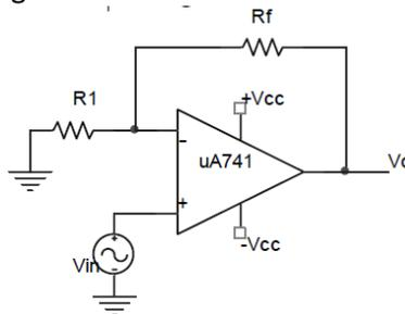
Figure 1 Non-inverting op-amp circuit
