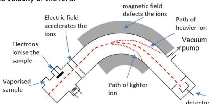
Figure 1 Schematic of a basic mass spectroscopy setup.
